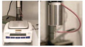
Figure 3. The test setup for measuring force required to make electrical contact through coating
